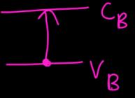
These are the polymers which have gap between valance and conduction band and cannot conduct electricity normally. They are doped with electron donor or electron acceptors to make them conducting.
